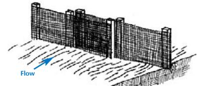
3. When joints are necessary, overlap ends for the distance between two stakes.
