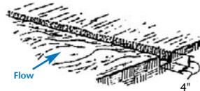
1. Excavate a 4" x 4" trench along the contour.
