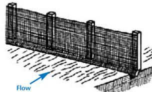
2. Stake the silt fence on downslope side of trench. Extended 8" of fabric into the trench.
