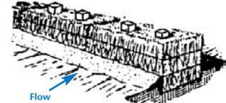
4. Backfill and compact the excavated soil.
