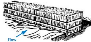
2. Place bales in trench with bindings around sides away from the ground. Leave no gaps between bales.
