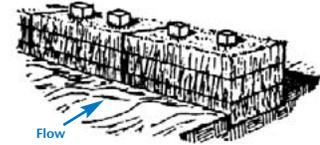
3. Anchor bales using two steel rebar or 2" x 2" wood stakes per bale. Drive stakes into the ground at least 8".
